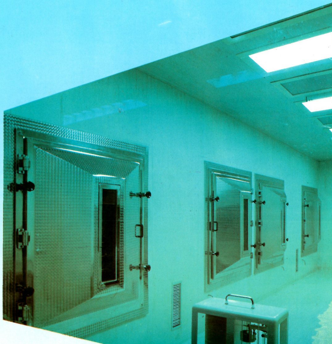
Impianti lato camera sterile View from the steril room side of freeze-dryer units
